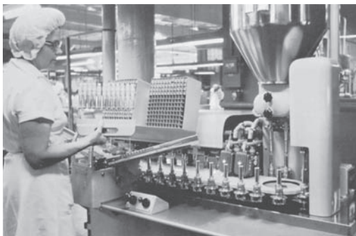
FIGURE 10.6 Arenco tube-filling machine automatically fills 125 tubes a minute with proper amount, tightens cap, orients each tube by electric eye so that label faces forward, then closes and crimps the end. (Courtesy of Eli Lilly and Company.)
