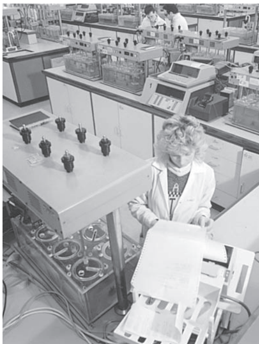
FIGURE 8.17 A modern computer laboratory dedicated to studies of drug dissolution from solid dosage forms. Included are Erweka dissolution baths, Hewlett-Packard computers, and Hewlett-Packard diode assay spectrophotometers. (Courtesy of Elan Corporation, plc.)
