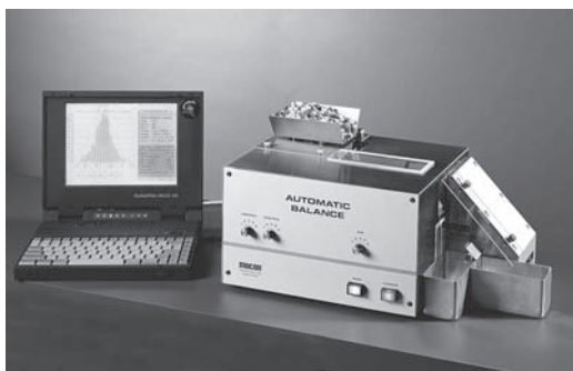
FIGURE 8.9 Automatic balance that weighs product and prints statistics to determine compliance with USP weight variation requirements for tablets. (Courtesy of Mocon Modern Controls.)
