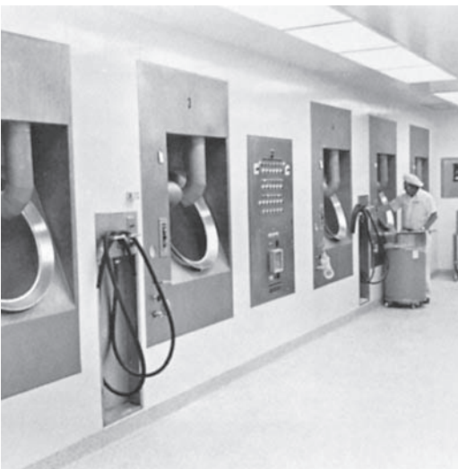
FIGURE 8.31 Modern tablet-coating facility. Air and exhaust ducts to assist drying are automatically operated from central board. (Courtesy of Eli Lilly and Company.)
