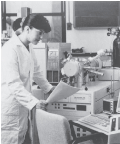
FIGURE 5.18 Computed gas chromatography mass spectrometry used in bioanalytical studies. Consists of Hewlett Packard Gas Chromatograph (Model 5890 A) and VG Mass Spectrometer (Model UG 12-250). (Courtesy of Elan Corporation, plc.)
