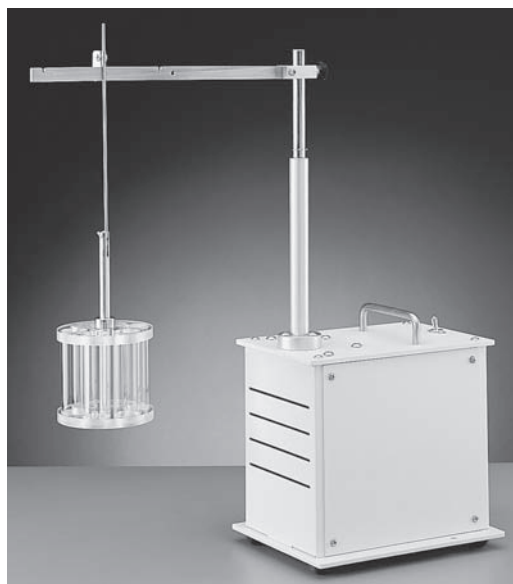
FIGURE 8.15 Tablet disintegration testing apparatus. (Courtesy of Varian Inc.)
