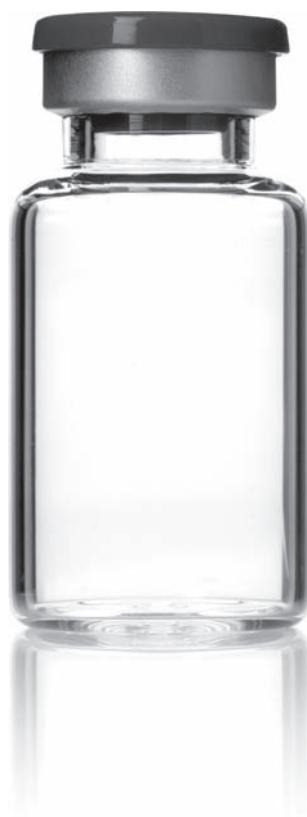
FIGURE 15.14 A typical vial for sterile injectable products, made from type I (borosilicate) glass. The rubber closure has been specially selected for compatibility with the product, desirable physical characteristics, and so on. The overseal holds the closure in place and provides ready access to the contents of the vial. (Courtesy of Hospira, Inc.)
