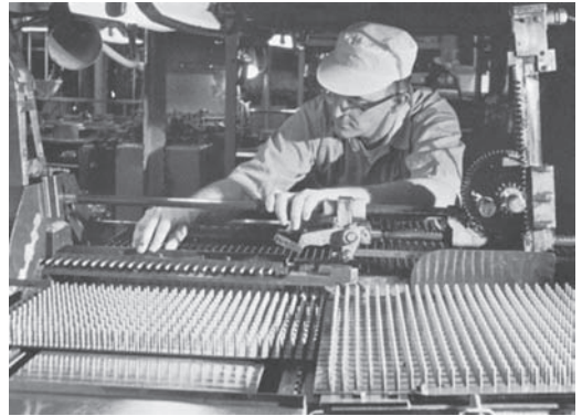
FIGURE 7.2 Body of capsules and their caps are shown as they move through an automated capsule-making machine. Each machine is capable of producing 30,000 capsules per hour. It takes a 40-minute cycle to produce a capsule. (Courtesy of Smithkline Beecham.)
