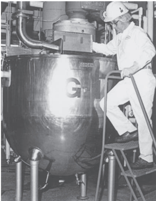
FIGURE 10.1 Creams and ointments in batch sizes up to 1,500 kg are manufactured in this stainless steel tank, which has counter sweep agitation and a built-in homogenizer. (Courtesy of Lederle Laboratories.)
