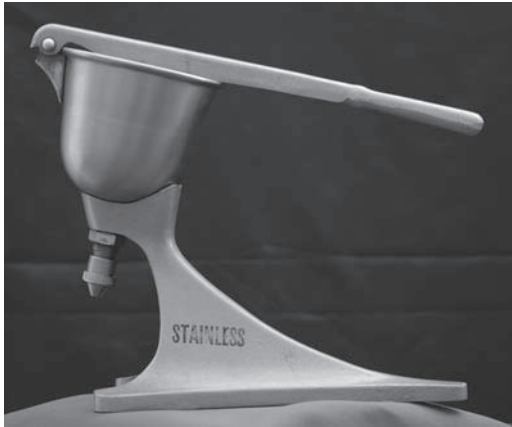
FIGURE 14.9 Laboratory preparation of an emulsion using a hand homogenizer.
