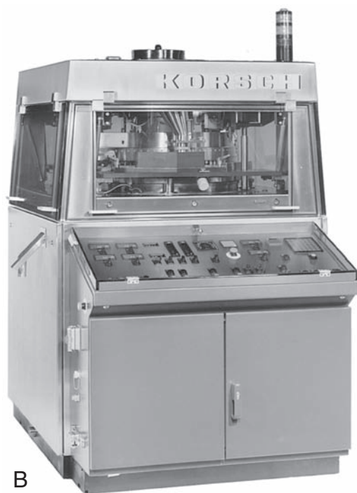
FIGURE 8.1 A. MiniTablet Press for development and small scale production (Courtesy of GlobePharma). B. High-performance double rotary tablet press. The Korsch PharmapressR has a maximum output of 1 million tablets per hour, but for continuous operation, it is generally run to produce 600,000 to 800,000 tablets per hour. (Courtesy of Korsch Tableting.)
