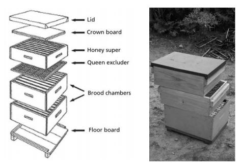
Fig. 6. The basic Langstroth hive. In the right-hand side of the figure, note the 'handles', or bars of wood for holding, on the supers and the scallop on the brood box. Handles make the whole business much easier
