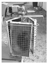
Fig. 21. Inside a motorized tangential extractor
