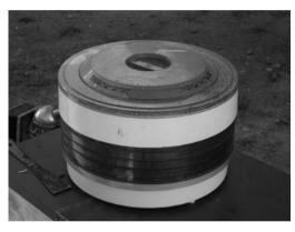
Fig. 33. A pollen drier heated by an element
