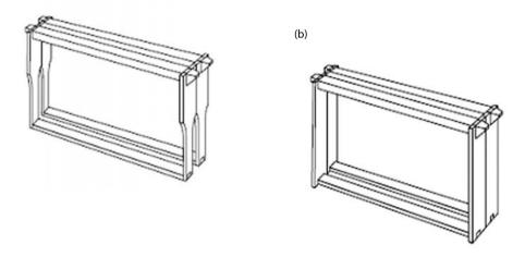
**Fig. 9.** Keeping frames apart: (a) the sides of the Hoffman Frame are scalloped to minimize contact with each other. This helps you to separate them yet also spaces them correctly; (b) Manley frames are straight down the edges, which facilitates uncapping
