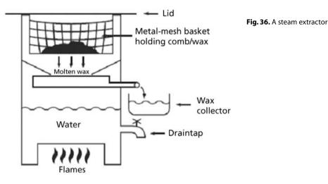
As you will see, you just need to place the old frames or the wax into the upper basket, close up, light up and wait for the wax to come pouring out. Make sure, however, that the container receiving the wax is pliable and large enough to hold a decent-sized block and, as soon as this is full, replace it with another one. You will need several of these containers on a good rendering day.
