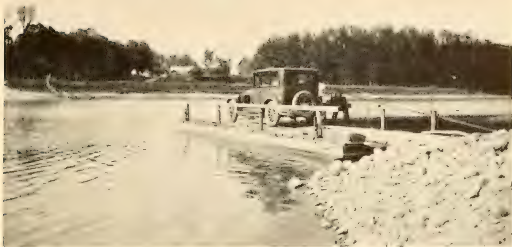
FIG. 179.—A ferry-float across the Grand River on the Six Nations Indian Reserve; it is propelled by the hands turning a toothed wheel over which passes a chain fastened to the shore, at either end.
