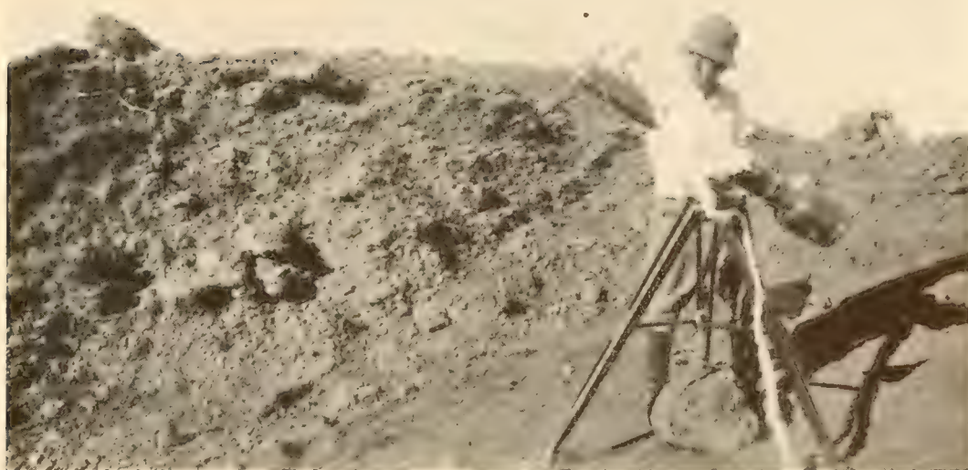
FIG. 4.—The new instrument at Fogo. Close-up view of Mr. Moore with the combination instrument for measuring atmospheric humidity, brightness of the sky, and intensity of solar radiation.
