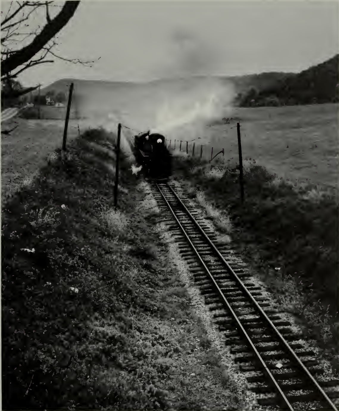
EBT LOCOMOTIVE #17, RUNNING LIGHT, NORTHBOUND ON THE NARROW-GAUGE RAILROAD'S MAIN LINE. Built in March 1918 by the Baldwin Locomotive Works in Philadelphia, Pennsylvania, the 163,500-pound steam locomotive is the second largest of the EBT's six Baldwin Mikados.
