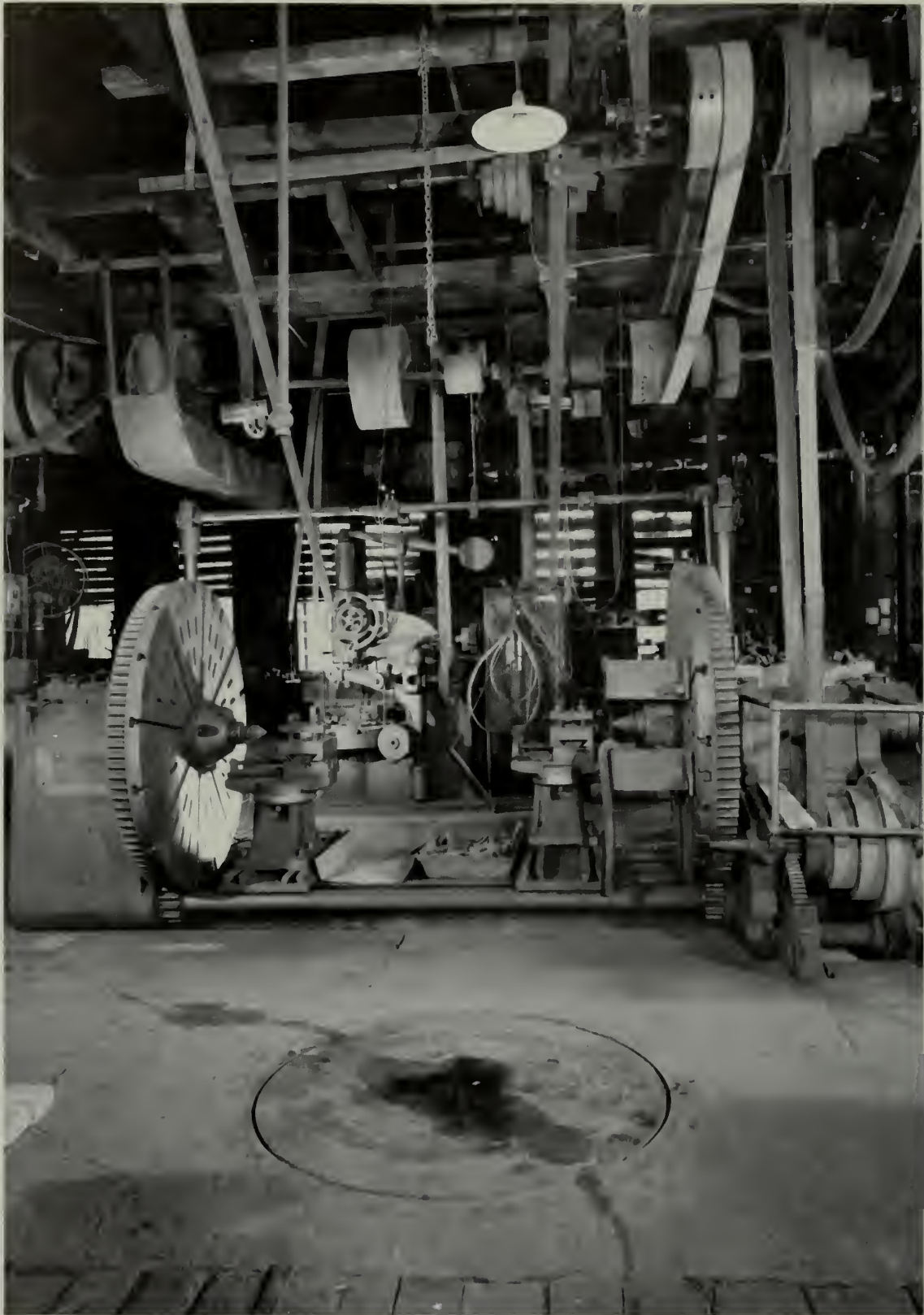
A WHEEL LATHE IN THE MACHINE SHOP. This massive 66-inch lathe was used to turn locomotive driving wheels and car wheels to restore their flanges and treads to round. The machine shop has no overhead crane, and all the work was manhandled from place to place. The small turntable in the cement floor directly in front of the lathe helped in manually turning wheelsets end for end.
