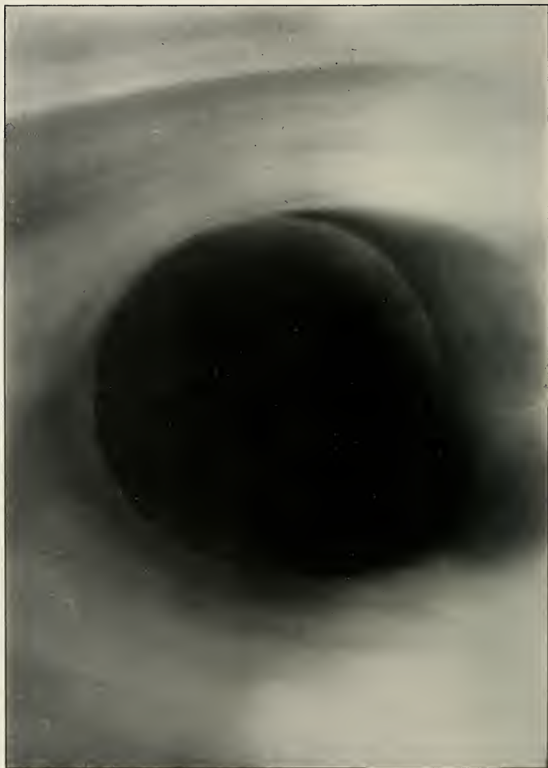
PHOTOGRAPH SHOWING FLOW OF AIR ROUND A CYLINDER IN MOTION.
