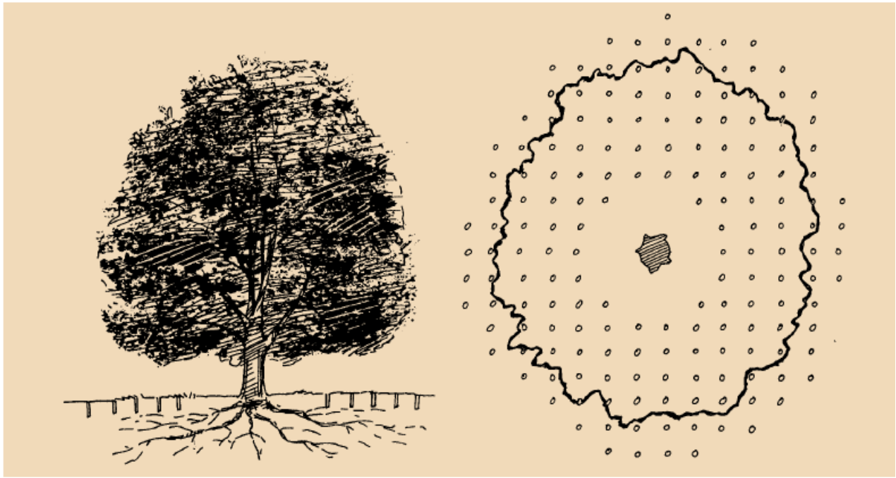
Figure 30. Vertical mulching can help repair compacted soils and help trees recover from root systems damaged by compacted soils and root removal.
